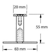
**DS 100** DEEP SECTION HANDRAIL & GUARDRAIL BRACKET CONCEALED WALL FIXING
